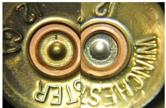
Fig 2. Single-barrelled test-fire on left; evidence shotshell on right.
