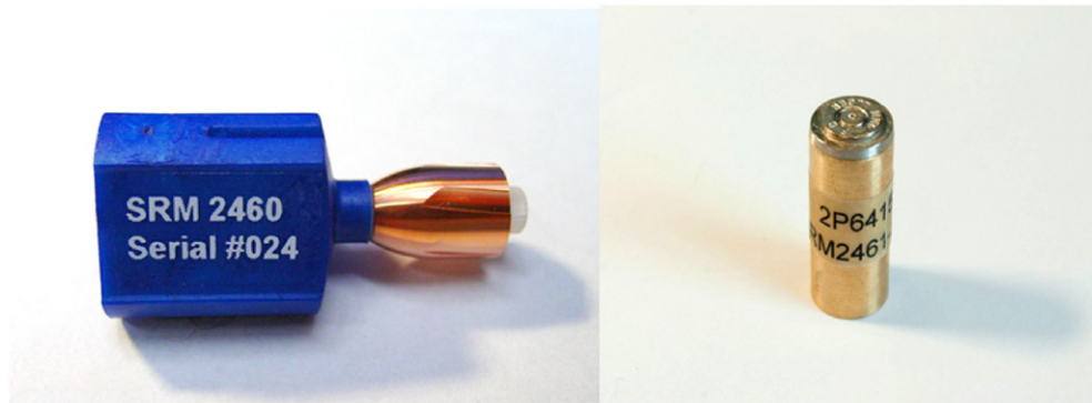
Figure 1. A SRM2460 standard bullet (left) and a SRM 2461 standard cartridge case (right).
