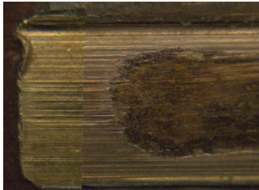
Identification based on individual characteristics from the land of a firearm barrel imparted onto the surface of a bullet
