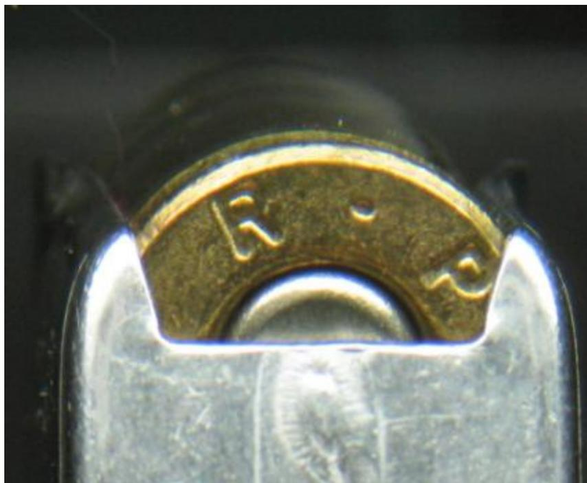
Cartridge loaded into the finished magazine
