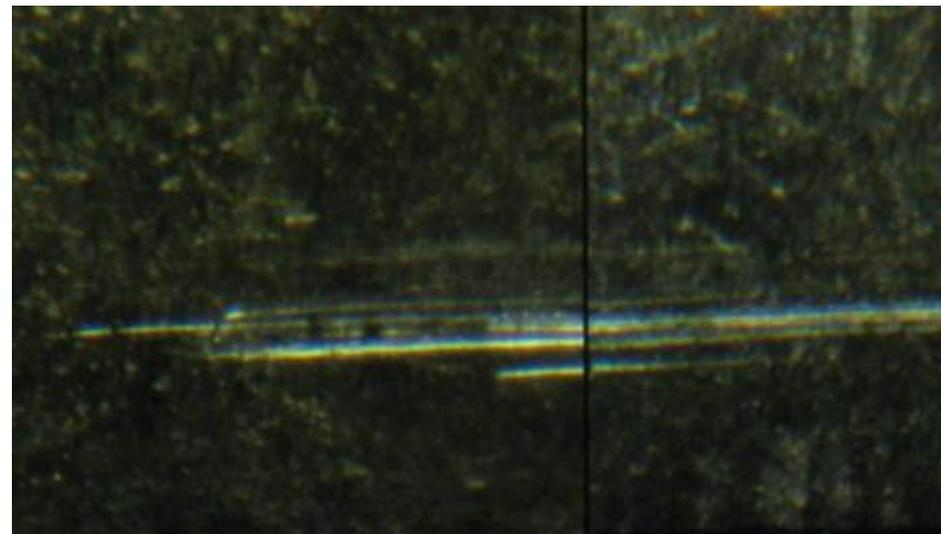
Photomicrograph of a magazine lip mark between two cartridges loaded into the same magazine
