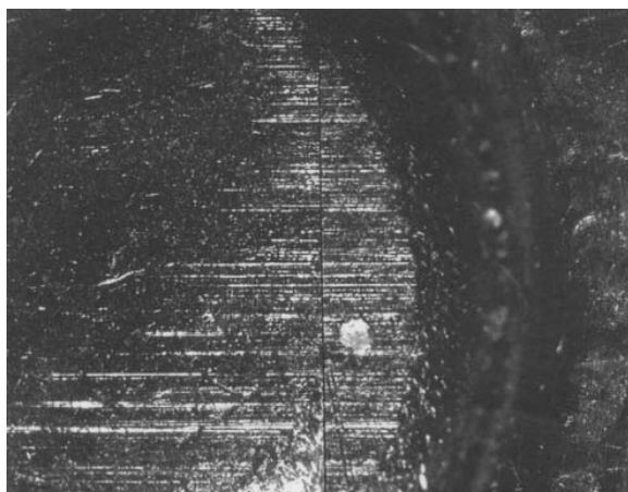
Figure 3: Some of the matching marks on the primers from the cartridge found in the suspect's car (left side) and one of the reloaded cartridges from the houseowner.
