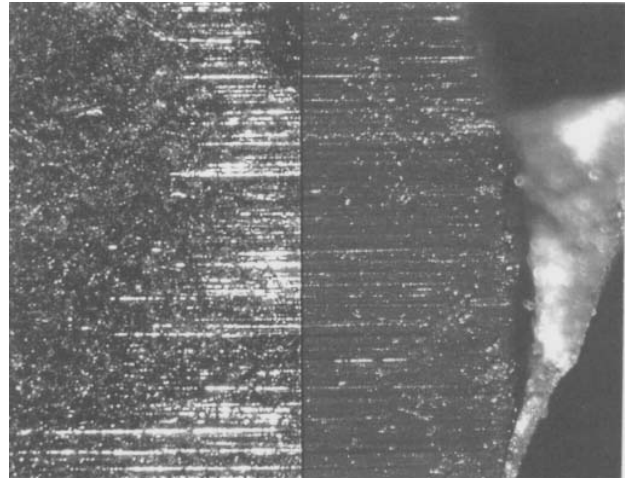
Figure 5: The matching marks between the cartridge from the suspect's car (left side) and the mikrosil cast from the primer punch head.
