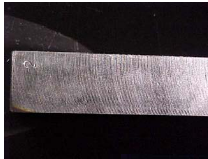
Photo 4: End milling toolmarks.
