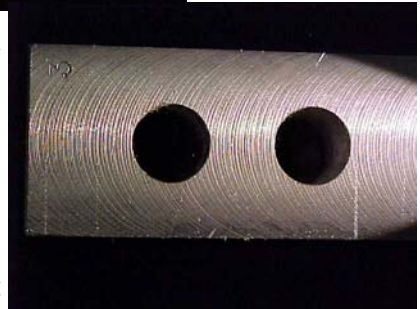
Photo 4: End milling toolmarks.
