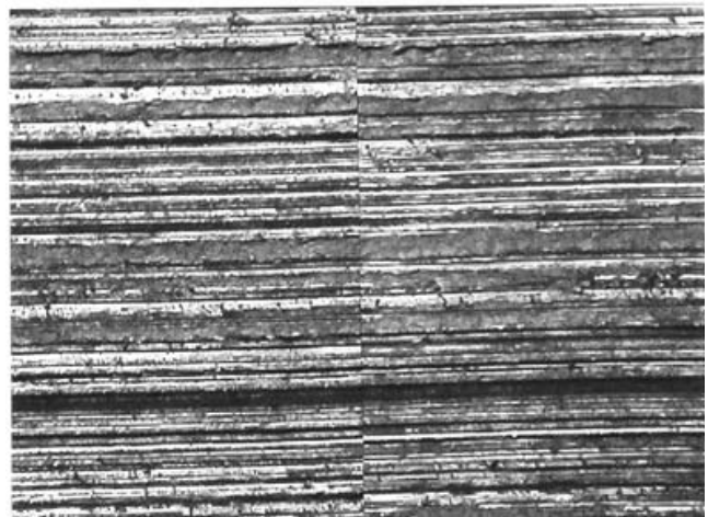
this stage in the manufacture process, these features are completely removed in the later finishing steps of manufacture (grinding and sharpening) and are not present on any final product tools. An example of true agreement of individual characteristics in finished product tools is evident in the comparison photograph of two toolmarks produced by side #2 of tool #2 from Tool Set #4. As evident, this particular tool readily reproduced its marks. (Figure 13). This is an example of a known-match.
