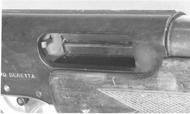
Figure 7: Ejector's cut-out in Beretta A390 shotgun.
