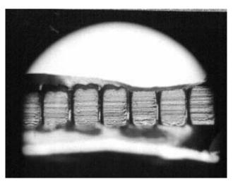
Microsil casts were made of the twenty-eight ejectors and taken back to the laboratory for further examination under our comparison microscope. Digital photographs were taken of the four Microsil casts, each with seven ejectors per cast, by placing the lens of the Nikon Coolpix 950 digital camera on the eyepiece of the microscope.
