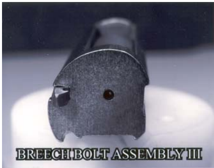
Figure 1: Granular Breech Face Marks
