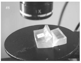
suggested the placement of a paper backer on each of the Mikrosil casts before they harden to assist labeling the casts.
