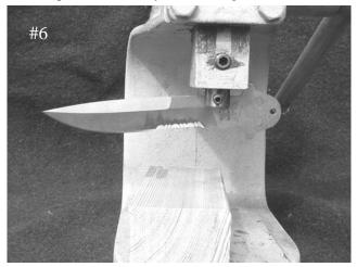
The cutting process was done with one knife and two groups of strips (numbers and letters) one set at a time to eliminate the possibility of co-mingling samples. Cuts were not made through the entire block to allow easier orientation to one another and to prevent drying.
