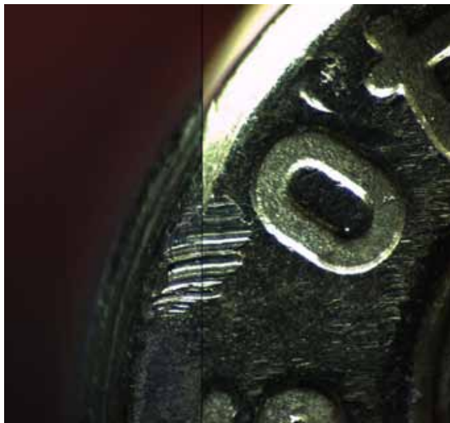
Photo #5: Example of marks below ejector mark – ID from Slide 10.
