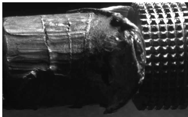
Figure 2: Land impression of one of the questioned bullets (nose at right), which is representative of the quality of rifling impressions observed on all of the questioned bullets.
