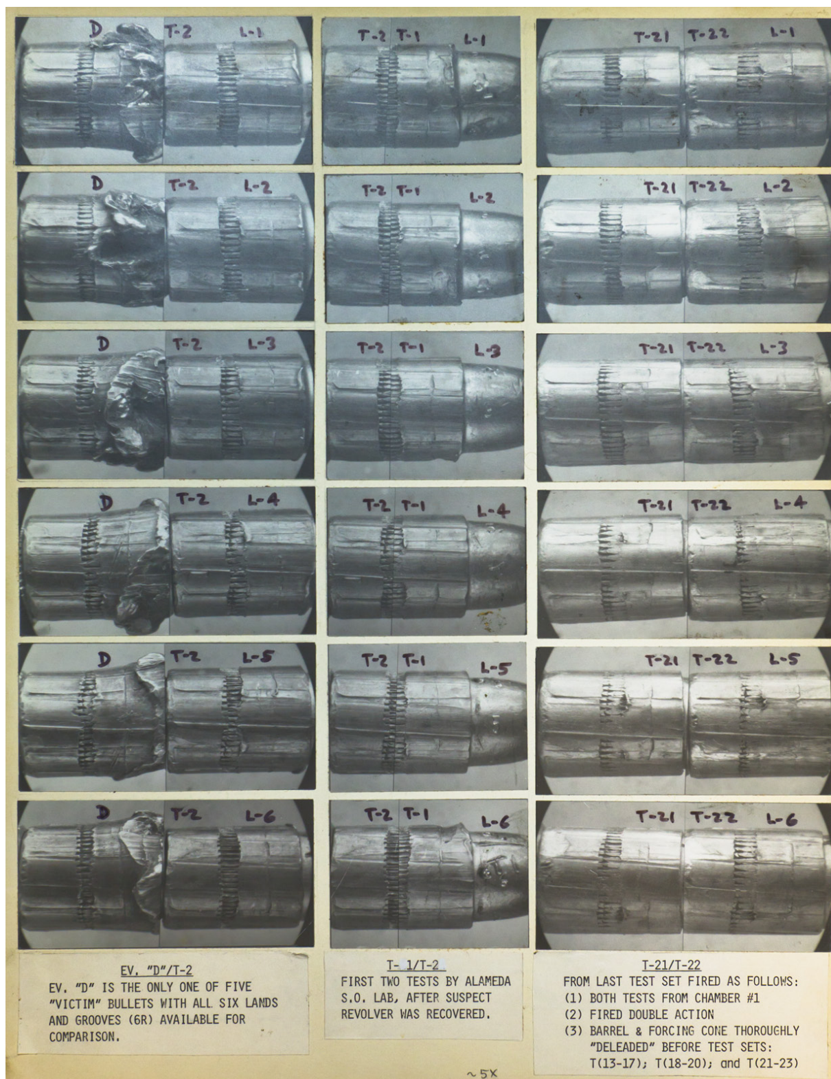
Figure 7: Biasotti's "Bald Bullet Board", used to summarize the microscopic comparisons he conducted. Note descriptions at bottom of each column of photographs. (Courtesy of J.E.M.)
