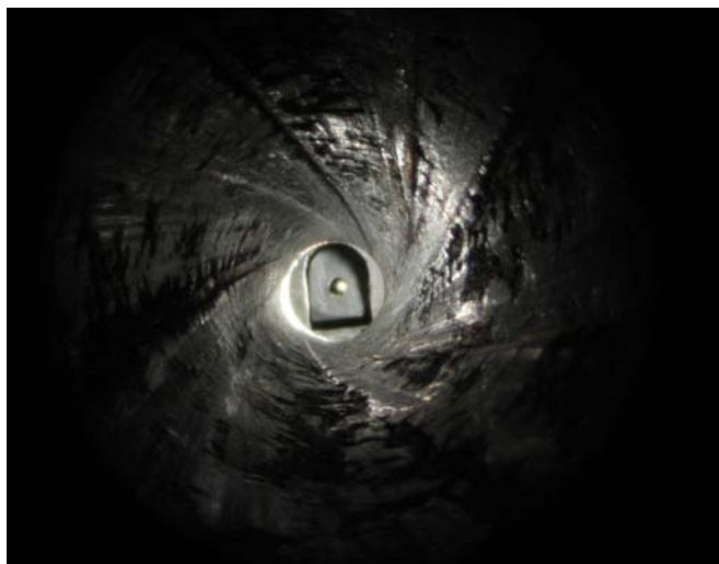
Figure 4: Additional photograph of bore, taken from a position closer to breech end with incident lighting to show surface texture of lead buildup.
