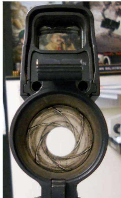
Figure 3: Rifled barrel of 40mm launcher
