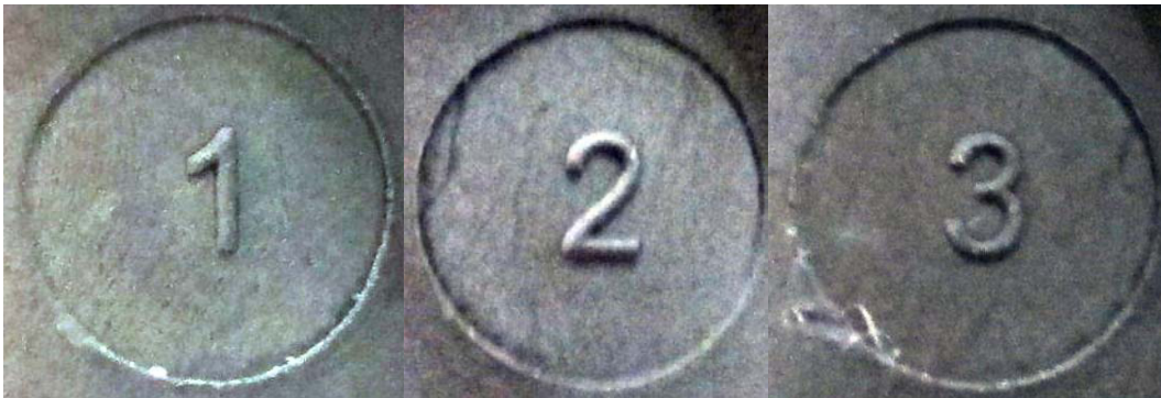
Mold marks from the multicavity mold
