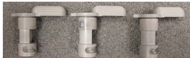
Three selector switches from same multicavity mold
