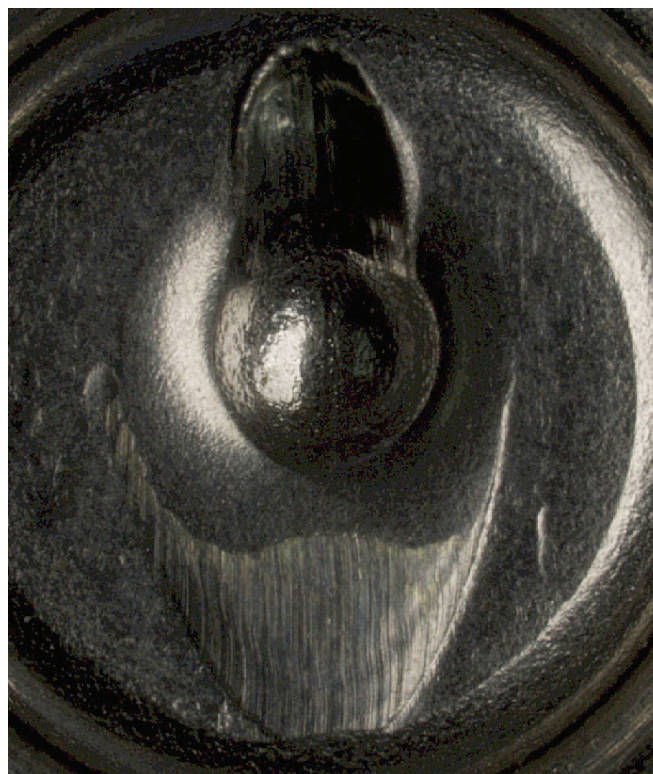
Figure 7: Fired cartridge case showing outline of weep hole & shear (40x)
