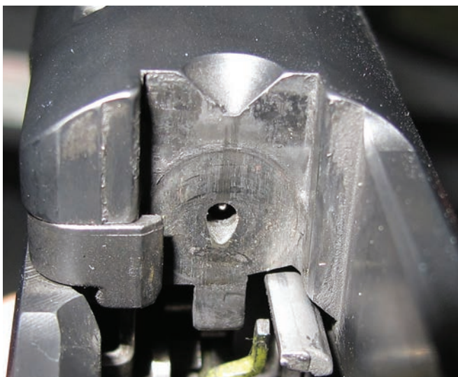
Figure 6: M&P breechface showing weep hole at base of firing pin aperture
