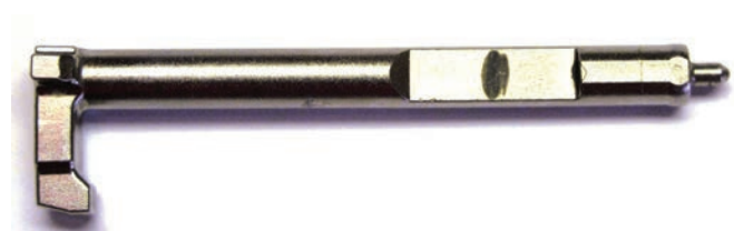
Figure 1: Overall of striker showing the black mark left from electropolishing
