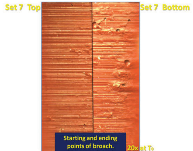
Figure 15: Top and bottom portions from a single pass of broach. Note that the stria have changed from beginning to end.
