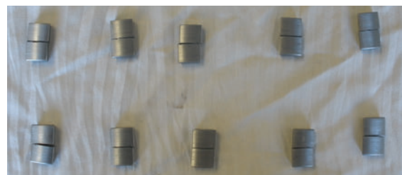
Figure 4: Demonstration of how workpieces were physically matched and designated as sets 1 - 10.
