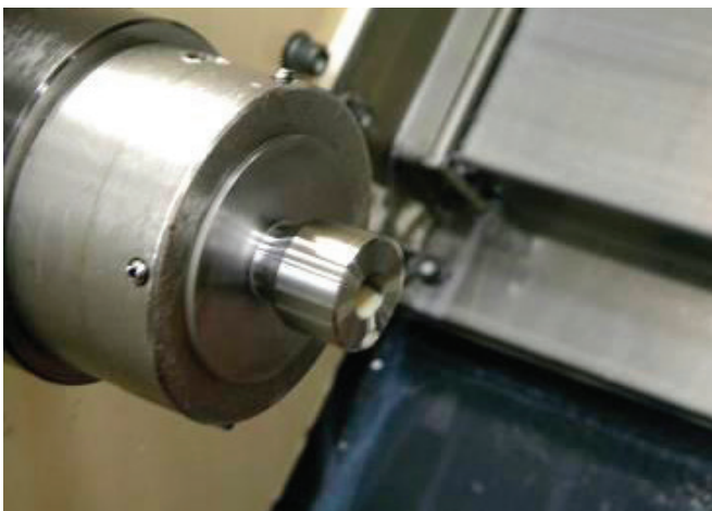
Figure 9: Reaming on the Back Side of the Barrel*
