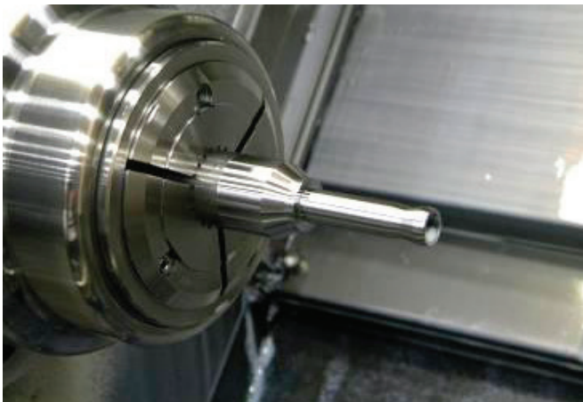
Figure 8: Barrel Blank after Turning and Drilling*
