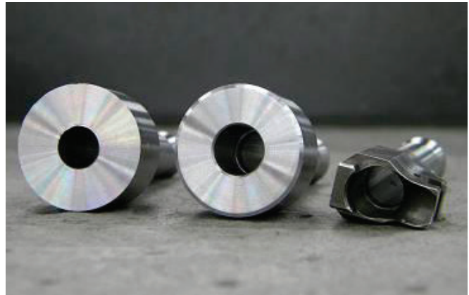
Figure 13: (Left to Right) Barrel from Turning to Drilling to Milling*
