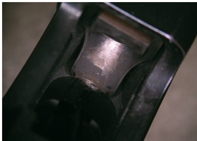
Figure 6: Ruger LCP – Barrel Position Rearward
