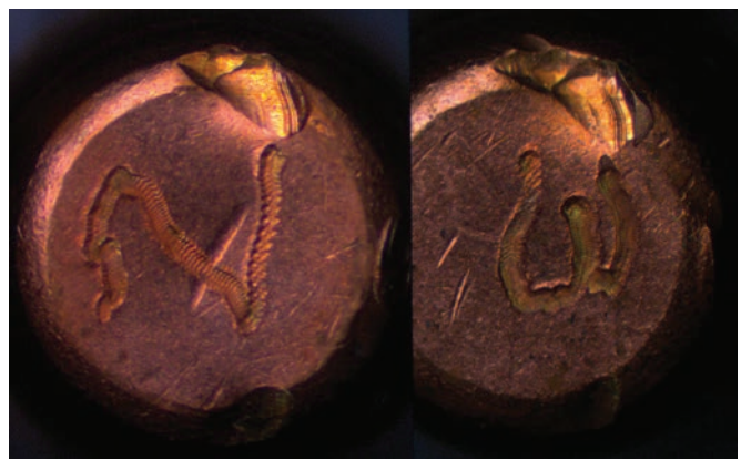
Figure 21: Feed Ramp Marks with Concentration on One Side (Group T9)
