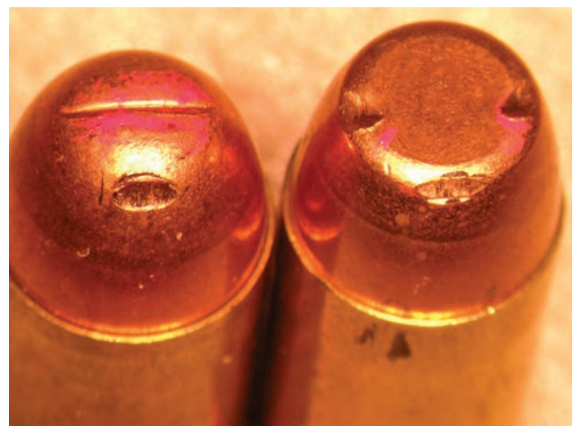
Figure 15: Ruger LCP Test Fires (fingernail polish transfer)
