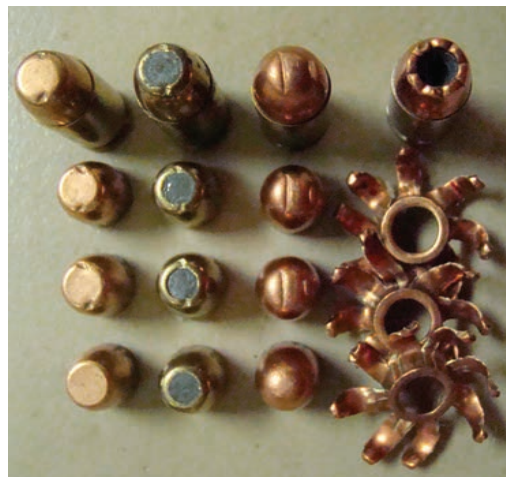
Figure 16: Ruger LCP Test Fires (Left to Right, Group A, C, B & D)
