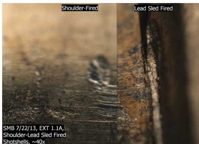
Figure 16: Agreement of marks from extractor 1.1A, fired from shoulder and lead sled (~40x)
