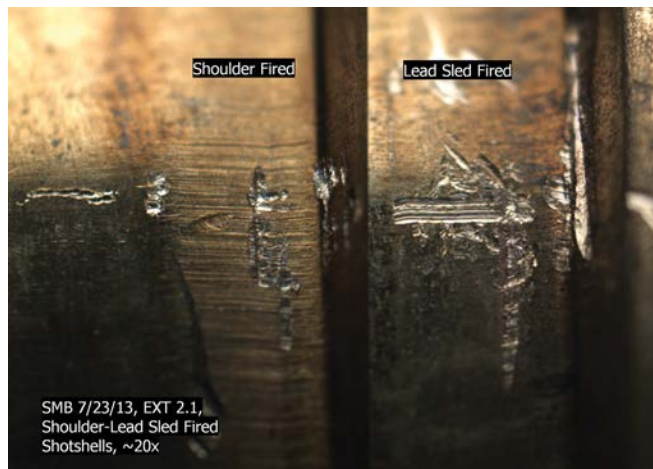
Figure 18: Quality of marks from extractor 2.1, fired from shoulder and fired lead sled (~20x)
