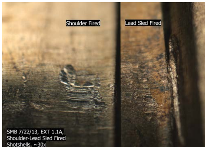
Figure 15: Quality of marks from extractor 1.1A, fired from shoulder and lead sled (~30x)
