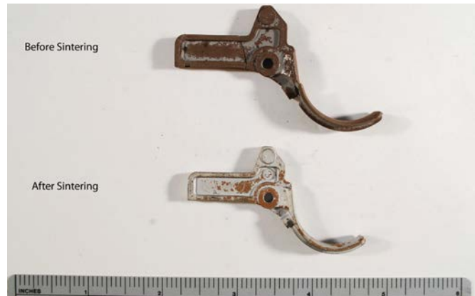
Figure 2: Remington triggers before and after debinding/sintering, displaying 15-20% shrinkage
