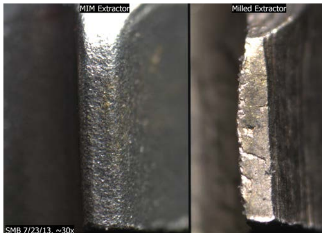
Figure 5: Surface of each extractor hook (~30x)
