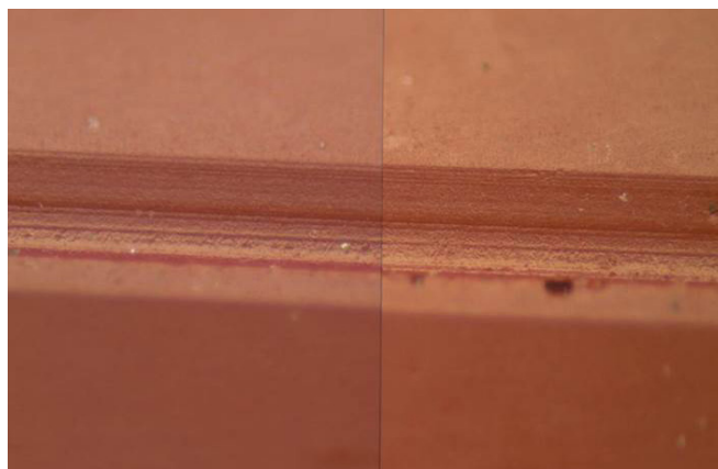
Figure 7: Subclass characteristics from two different barrels – Pattern A R2 (VDP913) (left) R2 (VDP968) (right)
