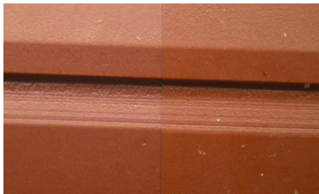
Figure 6: Subclass characteristics from two different barrels – Pattern B R1 (VDP913) (left) R1 (VDP968) (right)
