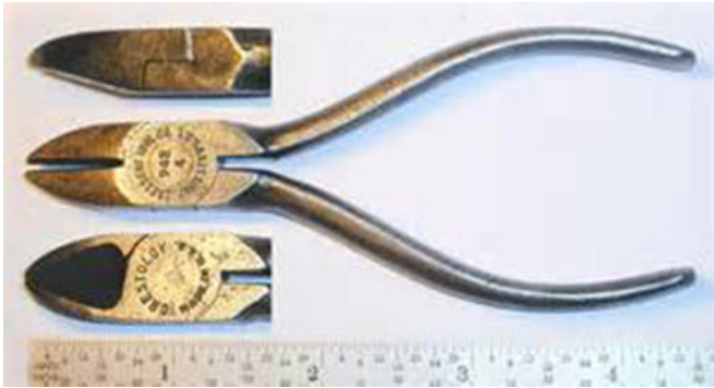
Figure 15A: Diagonal cutter with abutting blades employing pinching action (courtesy: wire2craft.com)
