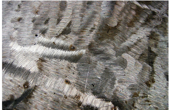
Figure 7A-2: Abrading toolmarks from a medium grit grinding wheel
