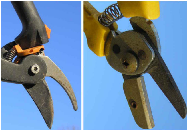
Figure 18A: Shearing blades, with bypass blade type on left and shear with designated anvil shear type on right (Courtesy: smallkitchengarden.net)
