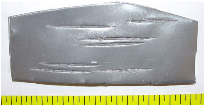
Figure 8B: Chopping impressions produced by hatchet in Figure 8A
