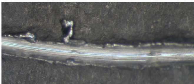
Figure 11C: Toolmarks produced from single point engraver at 30X magnification
