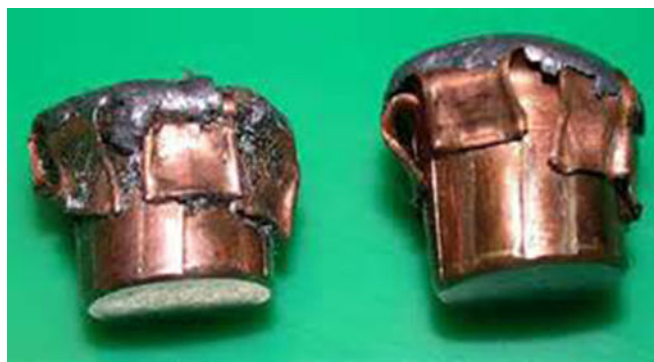
Figure 11D-2: Fired bullets with engraved impressions from firearm barrel lands
