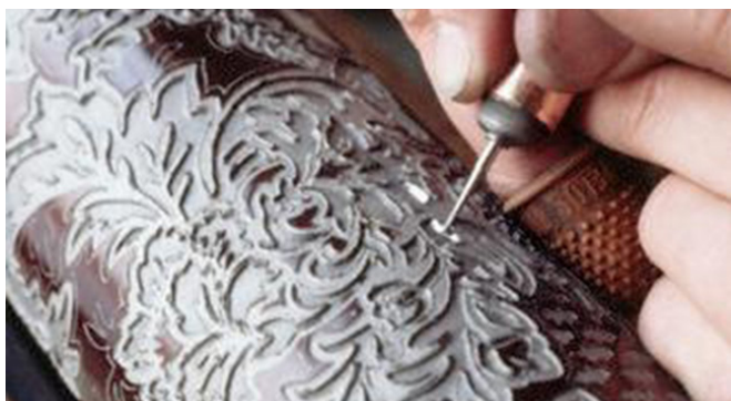
Figure 11B: Single point engraver where tool moves and workpiece is stationary (corporategifts4you.com)
