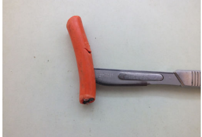
Figure 16A: Wire insulation pierced with a scalpel tip
