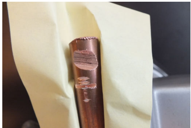
Figure 7B-2: Abrading toolmarks from coarse grit grinding or cutting disc. Note metal flow is even but striae are non-uniform
