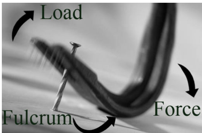
Figure 14B: Leveraging claw tool (pull) mechanics in removing nail (courtesy: republicanhour.com)
