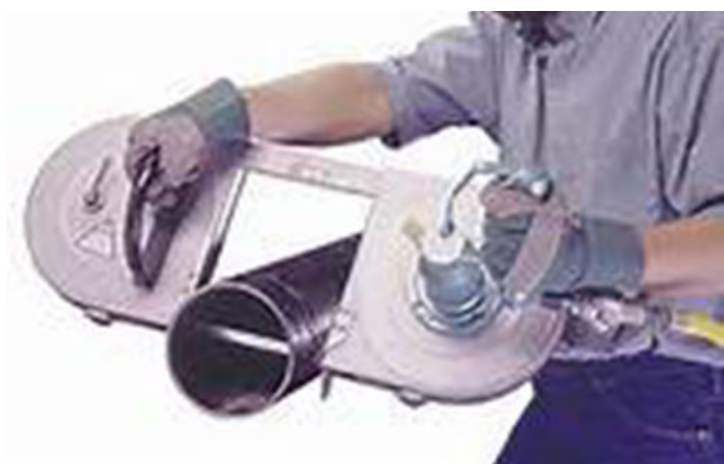
Figure 17C-1: Cutting pipe using a continuous cutting band saw (Courtesy: csunitec.com)
