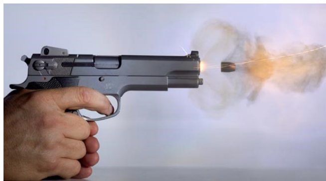
Figure 11D-1: Bullet being discharged and engraved by the lands of a firearm barrel where engraving tool (rifling in barrel) is stationary and workpiece (bullet) moves (courtesy: strangemilitary.com)
