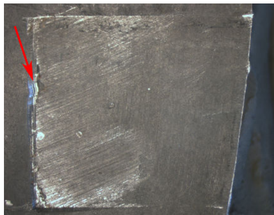
Figure 14D: Impressed type toolmarks produced by a flat leveraging pry tool blade. Note the striated sliding toolmarks produced by the pry end tip near middle of left edge
