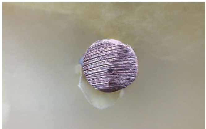
Figure 7C-2: Abrading toolmarks from coarse grit grinding disc. Note even metal flow is even but striae are non-uniform
