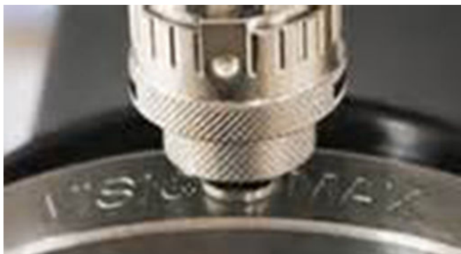
Figure 11A: Letters cut by single point engraving machine where workpiece moves and tool is stationary (courtesy: gtschmidt.com)
