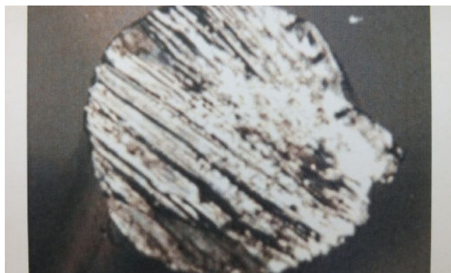
Figure 17B-2: Toolmarks produced by a reciprocating power saw
