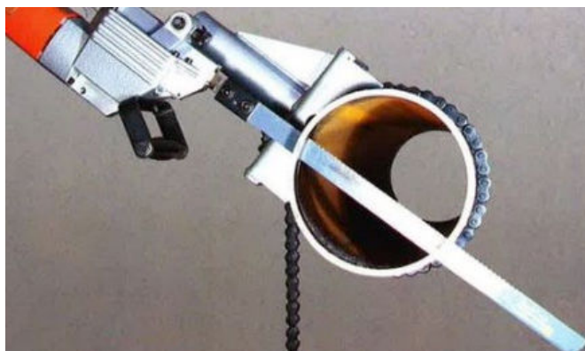
Figure 17B-1: Cutting by reciprocating power saw (Courtesy: csunitec.com)
