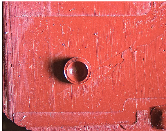
Figure 7: Cast of breech face of H&R Standard, 32 S&W caliber revolver
