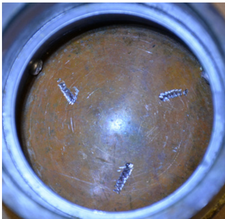
Figure 2: Toolmarks on the convex surface of an EFP liner
