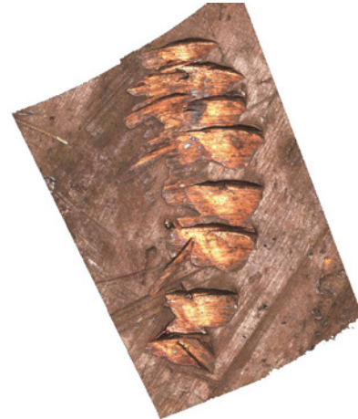
Figure 3: EFP toolmark (image taken using Alicona® Infinite Focus SI microscope)
