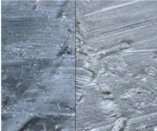
Figure 8: Corresponding detail in EFP toolmarks
