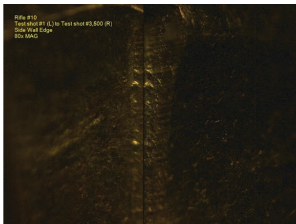
Figure 25: Rifle #10 Test 1 (L) vs Test 3500 (R) Side wall edge - 80x
