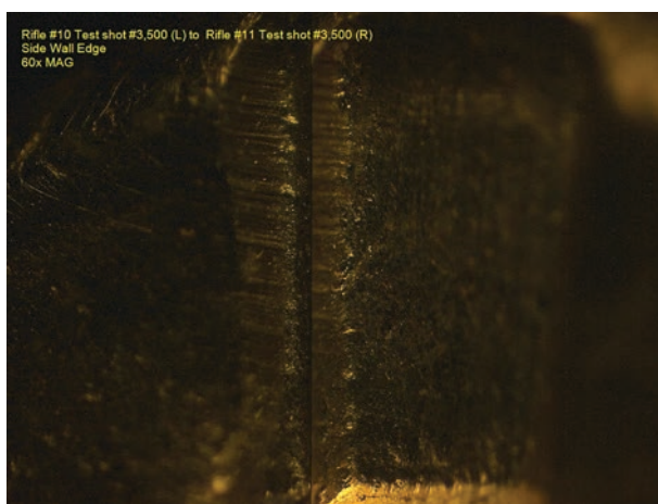
Figure 21: Rifle #10 Test 3500 (L) to Rifle #11 Test 3,500 (R) Side wall edge differences- 60x
