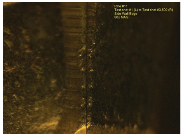
Figure 27: Rifle #11 Test 1 (L) vs Test 3500 (R) Side wall edge - 80x
