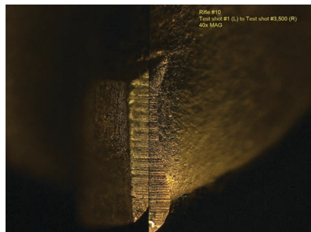
Figure 8: Rifle #10 Test shot #1 (L) to Test shot #3,500 (R) Side - 40x
