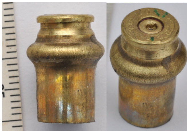
Figure 5: Swelling on a cartridge case discharged from a homemade submachine gun.
