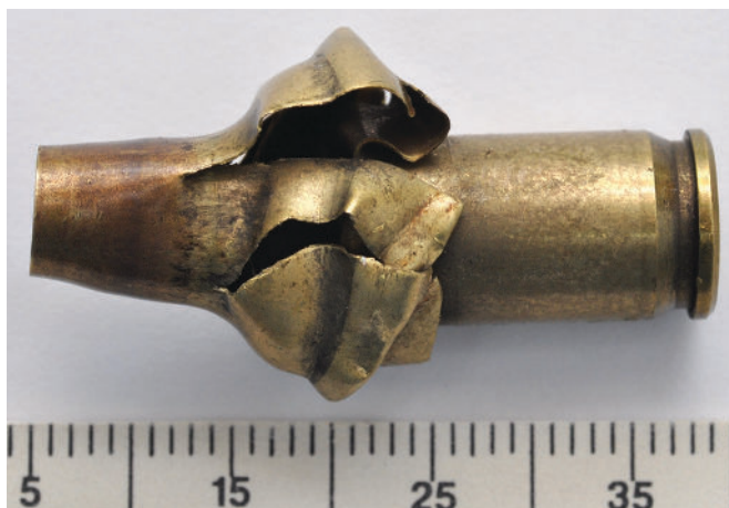
Figure 2: Ruptured cartridge case discharged from a primitive homemade firearm.
