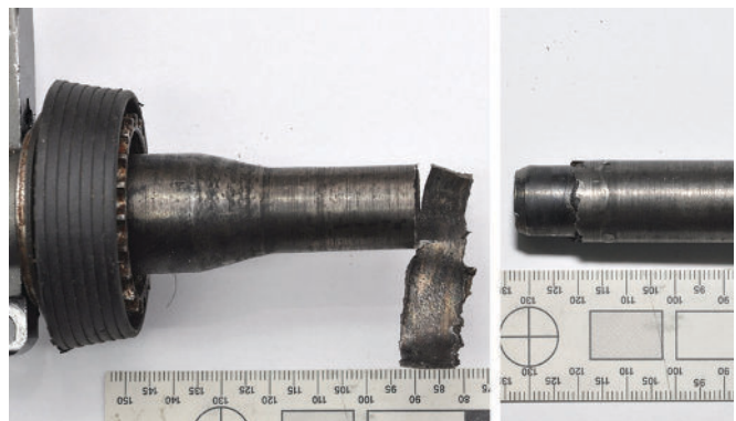
Figure 8: A barrel destroyed during shooting - the rifled barrel disconnected from the homemade chamber.
