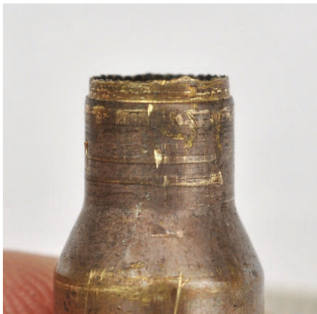
Figure 7: Marks on the cartridge case mouth imprinted from the connection between the homemade chamber and the rifled barrel.
