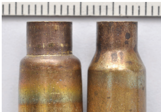
Figure 3: Cartridge cases in caliber 5.56x45 mm discharged from a homemade firearm (left) and from an original, correct caliber (right) chamber.
