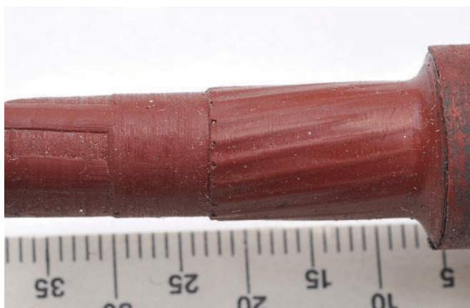
Figure 15: Cast of the chamber with the grooves, freebore and homemade rifling.
