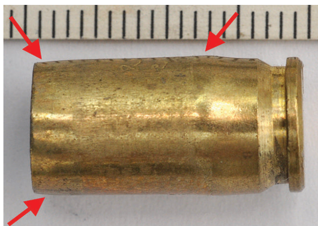
Figure 4: The deformation on a 9mm Luger cartridge case discharged from a homemade firearm.
