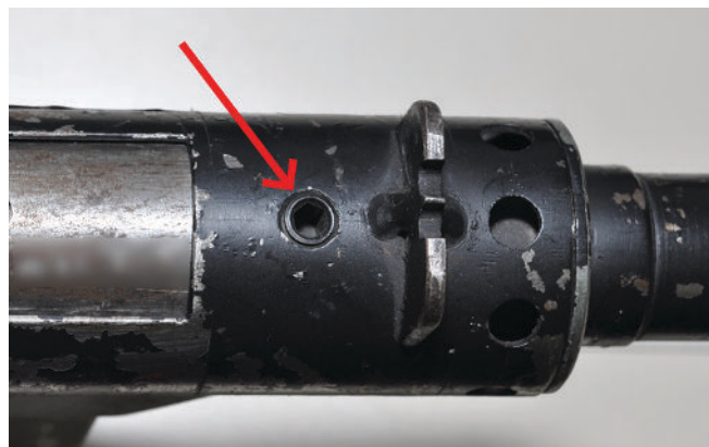
Figure 10: Barrel retaining screw in a homemade submachine gun.
