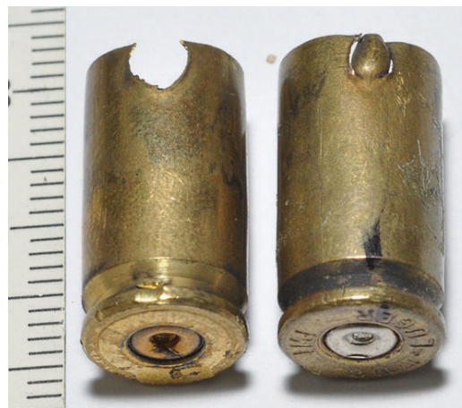
Figure 9: Perforation in the front part of cartridge cases made by a barrel screw hole of a homemade submachine gun.
