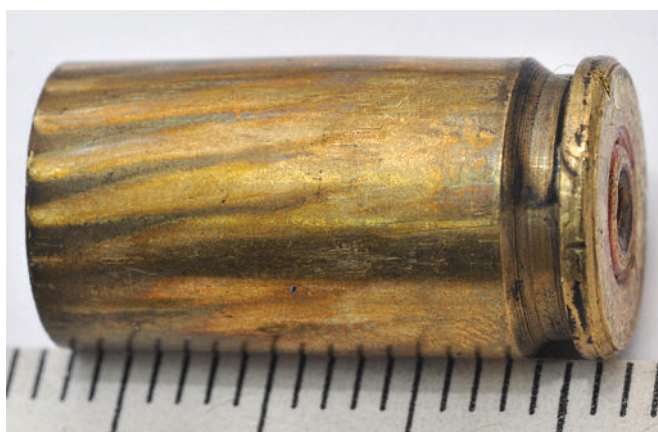
Figure 16: Marks of spiral grooves in the chamber of a homemade submachine gun.
