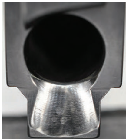
Figure 4: Feed ramp with grinding or honing marks.
