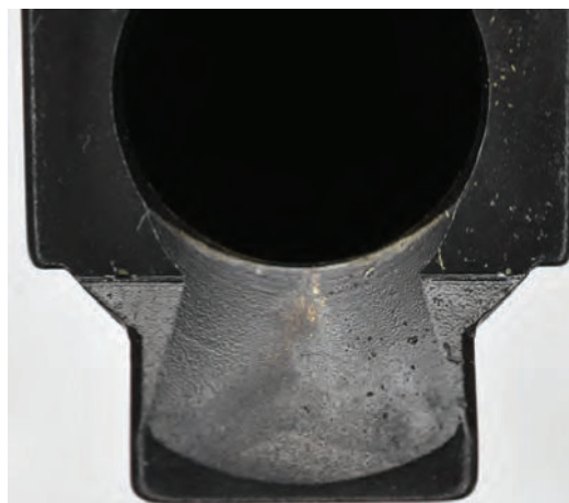
Figure 5: Feed ramp with granular appearance.
