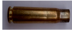
Figure 7: Deep Smile found on fired cartridge case B58.
