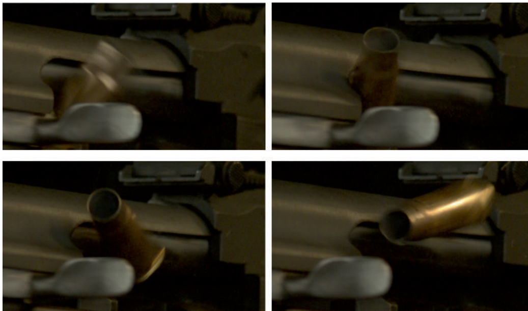
Figure 1: As the fired cartridge case is ejected from the firearm it strikes the edge of the dust cover creating the dust cover impact mark (slap mark) near the mouth of the fired cartridge case.
