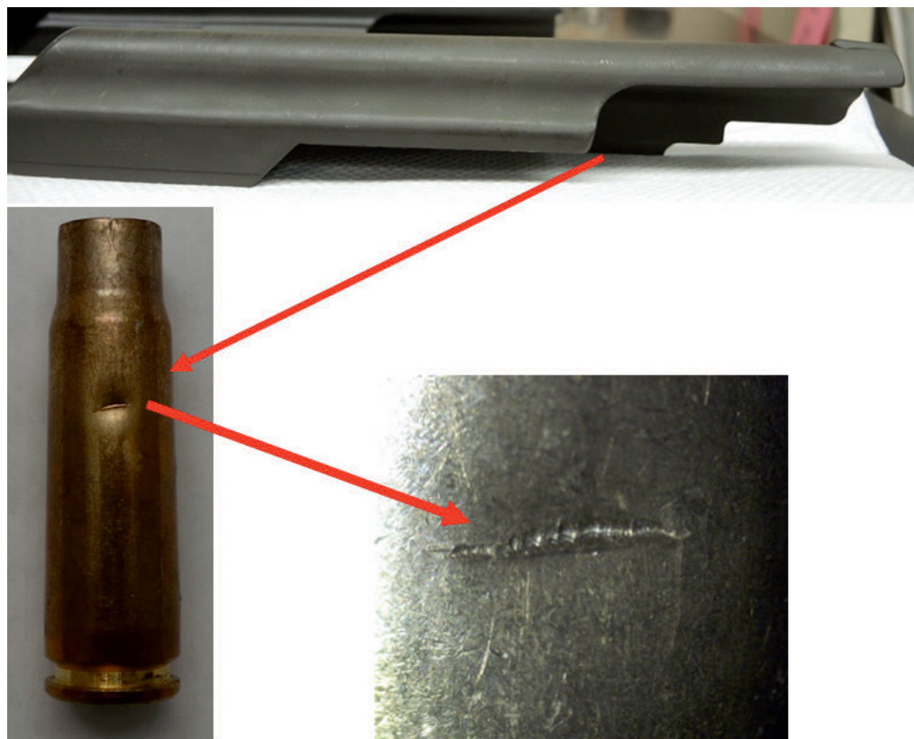
Figure 2: When a fired cartridge case is ejected and hits the dust cover, unique markings on the dust cover are imparted onto the fired cartridge case, sometimes referred to as 'slap marks' or dust cover impact marks. These marks viewed microscopically can be useful in making identifications between cartridge cases.
