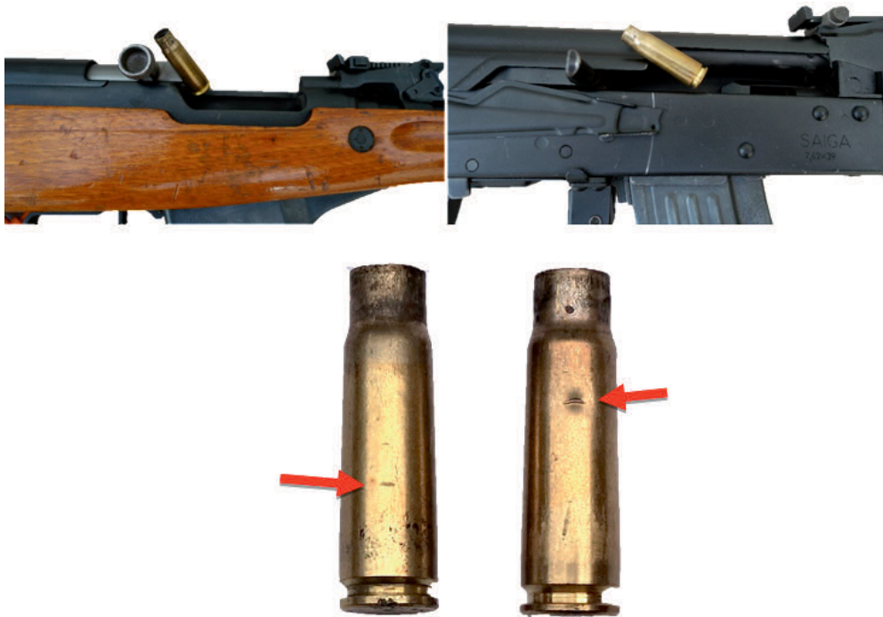
Figure 3: Characteristics of dust cover impact marks (slap marks) found on SKS-type rifles (left) and AK-type rifles (right).
