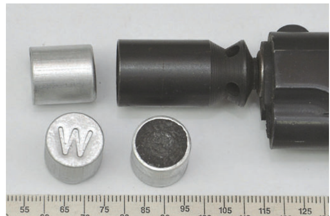
Figure 9: The flare adapter assembled to the pistol and flares
