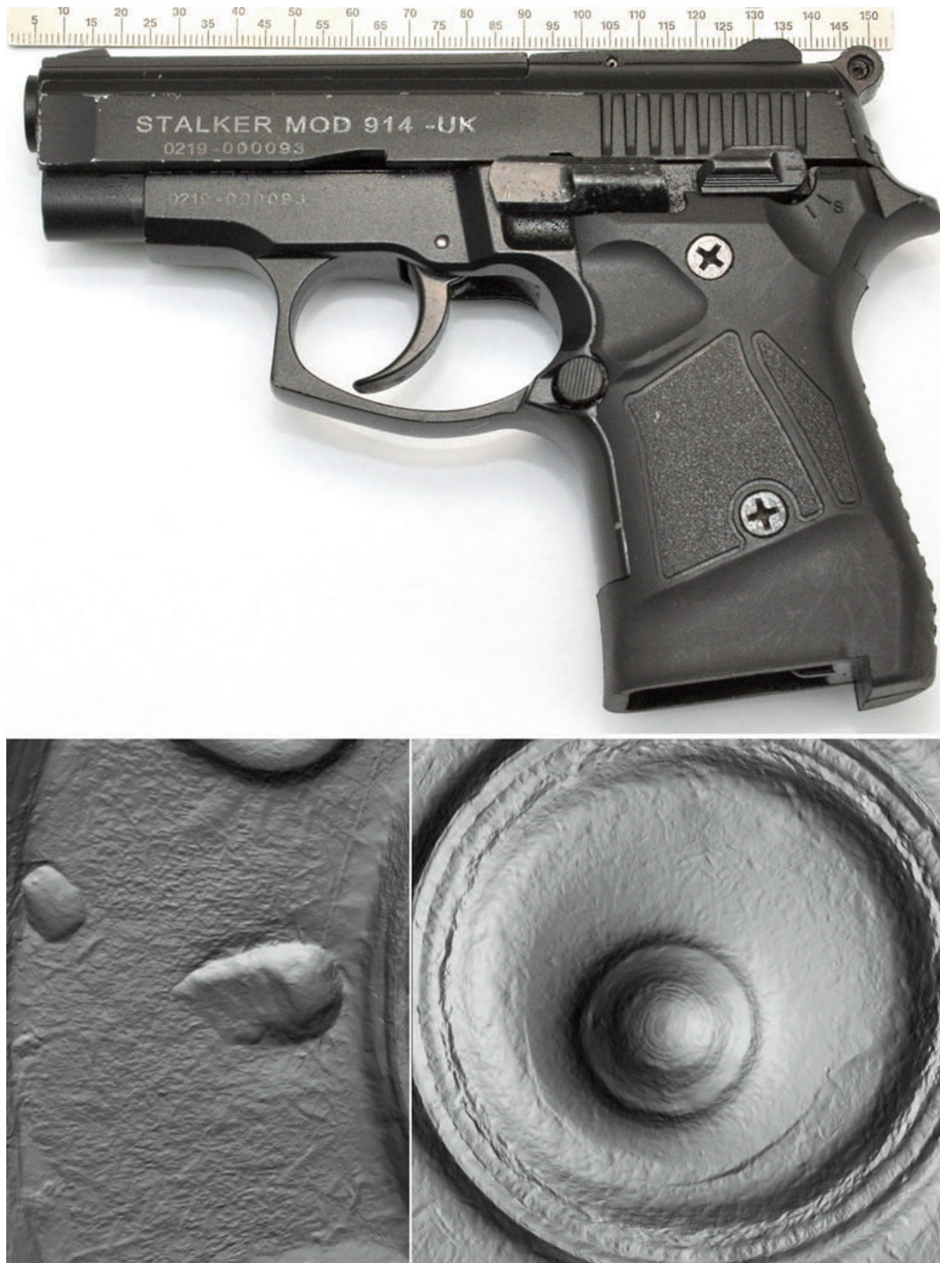
Figure 19: Stalker 914-UK and the examples of its class characteristics (ejector mark shown in the lower left and firing pin impression shown in the lower right)
