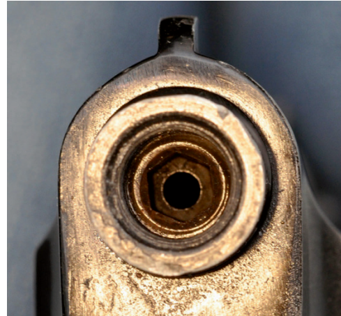
Figure 8: The construction element in the barrel of Ekol Firat Magnum gas pistol which prevents projectile shooting (the muzzle end view)
