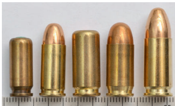
Figure 5: Calibers from left to right: 8 mm K (8 mm Knall), 32 Auto (7.65x17SR), 9 mm PA (9 mm P.A.K), 380 Auto (9x17), 9 mm Luger (9x19)
