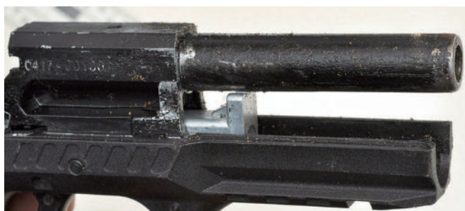
Figure 10: Blank pistol Stalker 4918-UK in which the barrel is replaced by a homemade part
