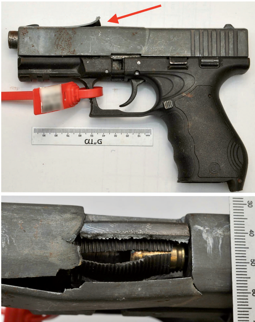
Figure 15: The catastrophic failure in a converted pistol with a homemade barrel
