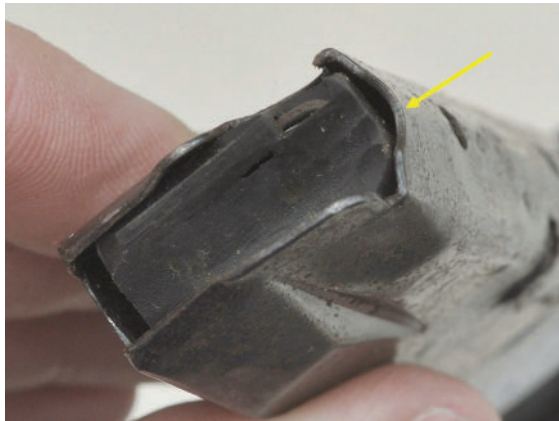
Figure 14: The modification of the magazine for loading cartridges with bullets
