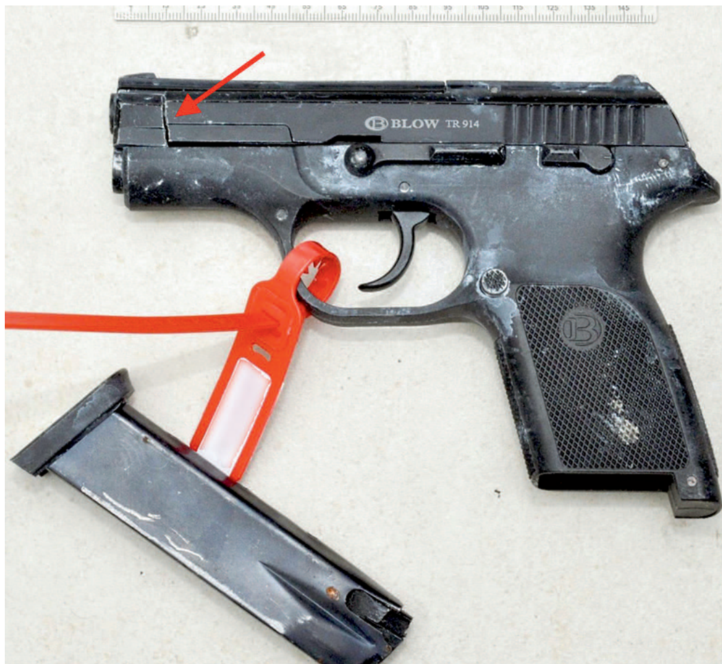
Figure 17: The catastrophic failure in a converted pistol (arrow pointing to the crack)
