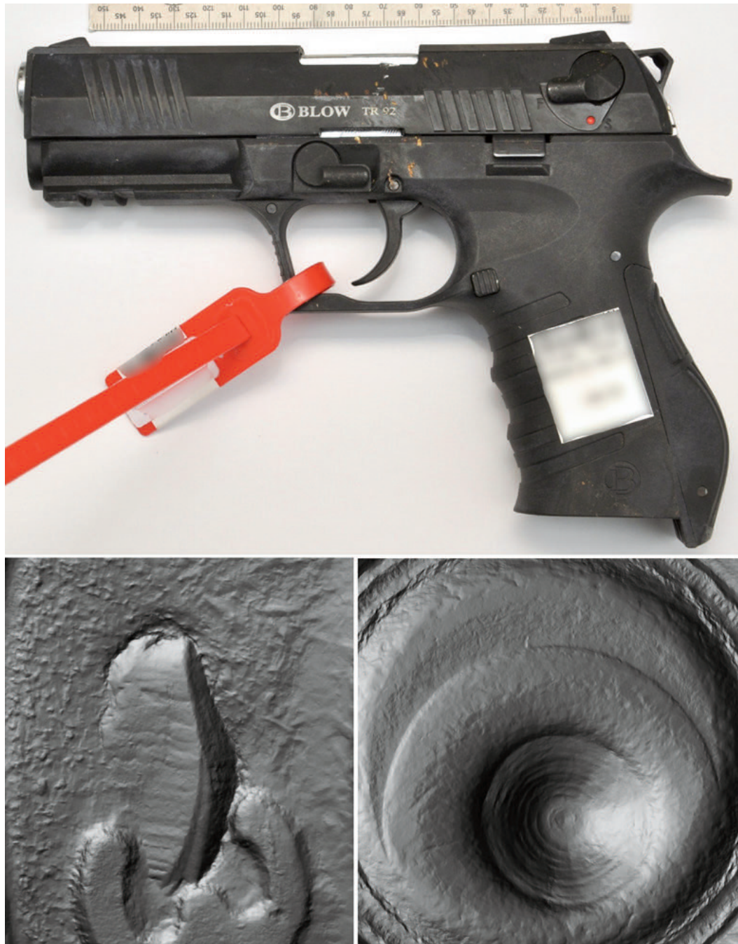
Figure 18: Blow TR92 and the examples of its class characteristics (ejector mark shown in the lower left and firing pin impression shown in the lower right)
