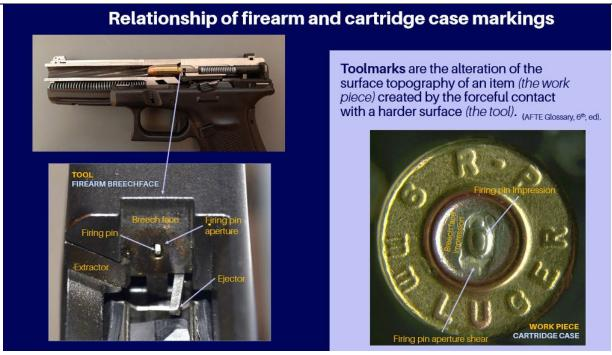
The working edges of tools, which include components of firearms that contact ammunition, generally consist of some type of hard material, such as steel, to ensure strength and durability of the tool while work pieces are generally made of softer materials (ammunition metals
