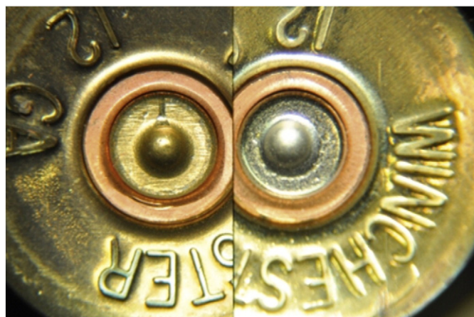
Fig 2. Single-barrelled test-fire on left; evidence shotshell on right.
