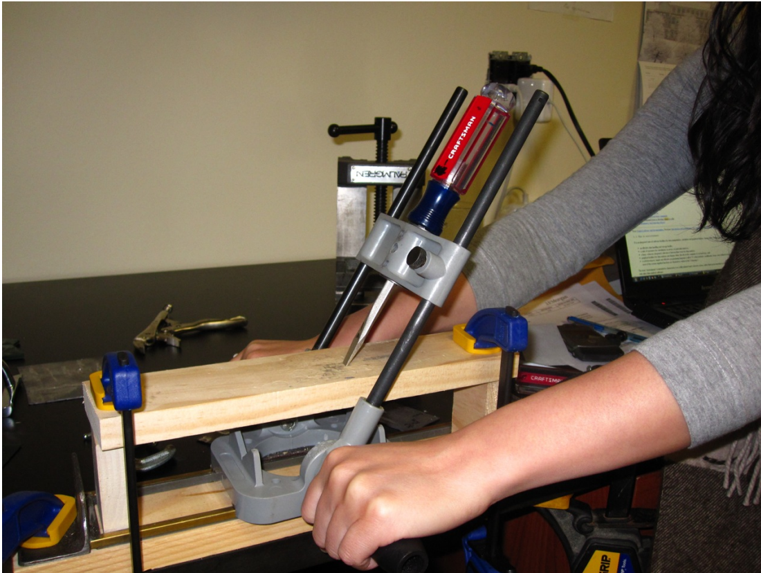
FIGURE 7. Tool holding jig for generating striation patterns on any media.
