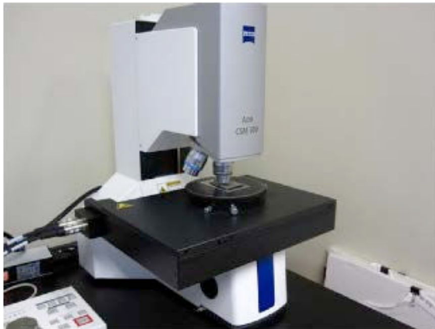
FIGURE 8. Zeiss Axio CSM 700 Confocal Microscope. Photograph courtesy of Peter Diaczuk.
