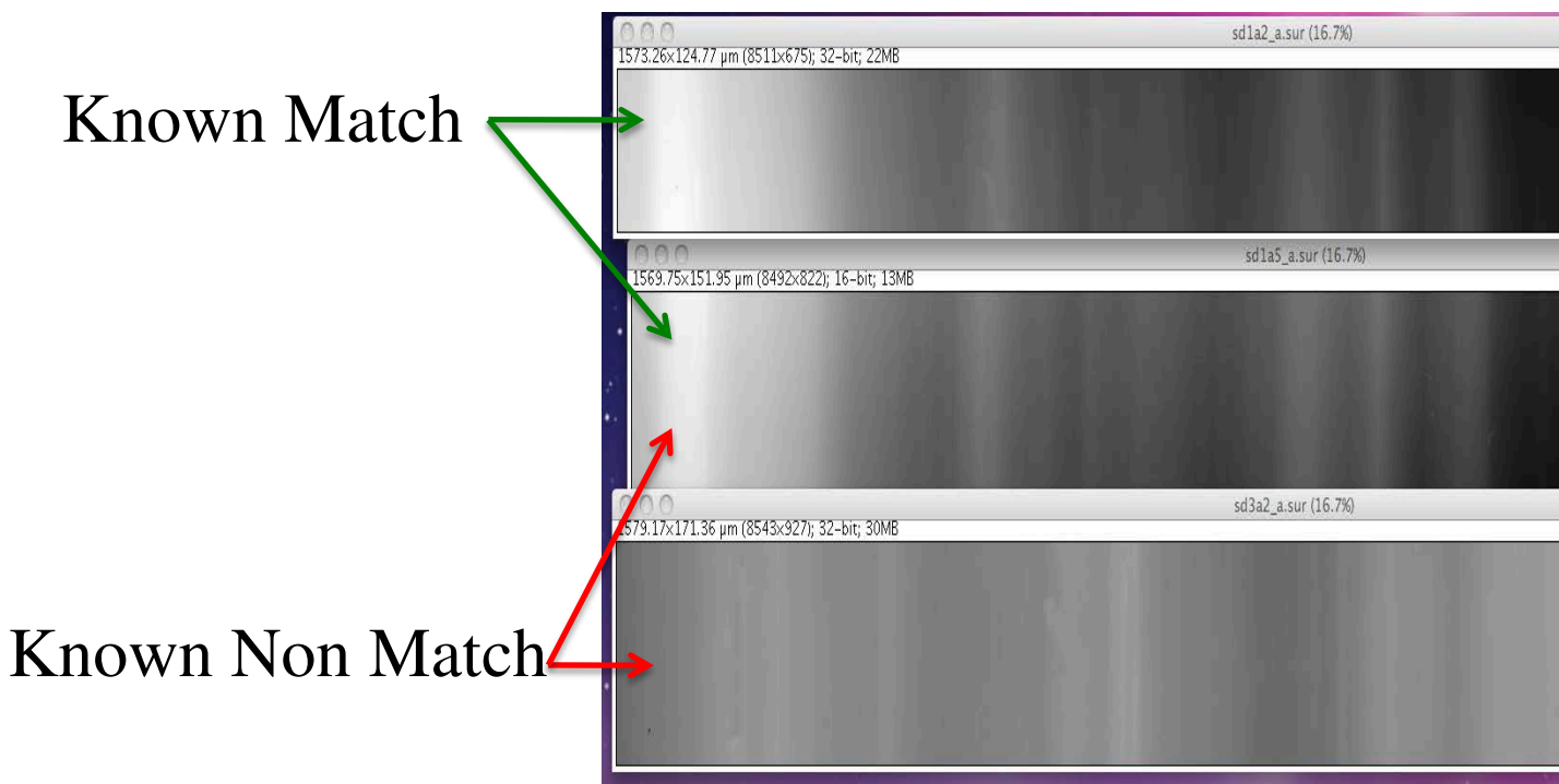
FIGURE 38. Topographies of three screwdriver striation patterns (two screwdrivers), shown in grey levels.
