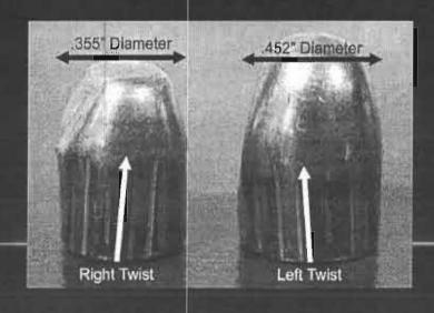
· Subclass characteristics are those shared by a subset of the previously defined population, and generally originate in the production phase. Examples are striations (scratches) imparted to work pieces during reaming, broaching, forging, blanking, etc.
